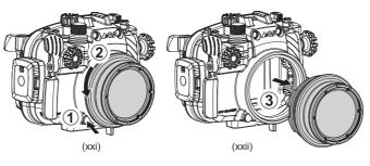
c. To install the Port Lens, align the Alignment Marks on the Lens Port and the Housing Body and then push the Lens Port completely down into Housing Body(fig. xxiii). Rotate the Lens Port clockwise until a "Click" sound is heard. When the Port Release Button is no longer depressed, the Lens Port is properly installed and locked(fig. xxiv)
