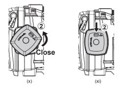
Once the camera is installed and housing is closed, turn on the power of the camera and make sure all housing controls and lens gear function properly. Check that the Optical Flash Trigger is functioning with the external slave strobe(s).
