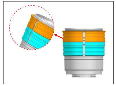
2 Insert the plastic C-ring for focus gear as shown and place it over the lens and plastic C-ring for zoom gear.
