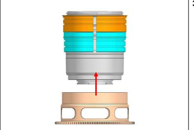
3. Insert the focus gear on a plastic C-ring for the focus gear until it reaches the flange of the plastic C-ring.
