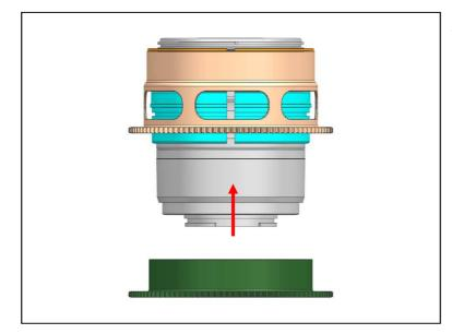
4. Insert the zoom gear on a plastic C-ring for the zoom gear until it reaches the flange of the plastic C-ring.
