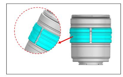
1. Insert the plastic C-ring for zoom gear as shown and place it over the lens.
