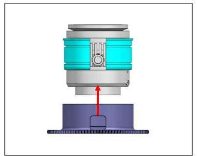
2 Insert the N1855AFP-Z Zoom Gear on the plastic C-ring until it reaches the flange of the plastic C-ring.
