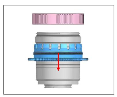
2 Place the Locking Ring over the gear and plastic ring, and screw it into the thread on the gear.
