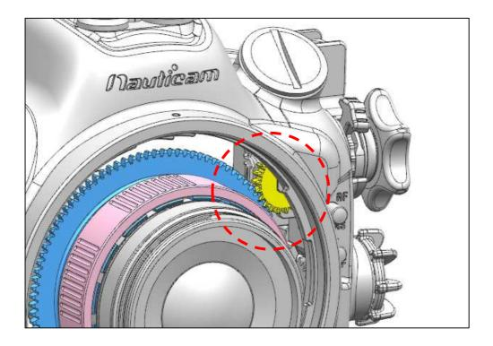
1. The CR1530-Z Zoom Gear can be controlled by zoom/focus knob of the housing.
