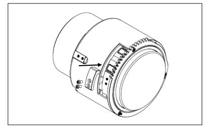
6. Align and tighten the screws with the Macro switch block pressing on the lens MACRO button.
