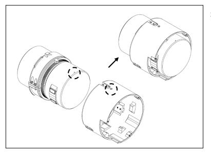
3. Align the alignment index on zoom gear tube with the red dot on the lens and insert the tube onto the lens.
