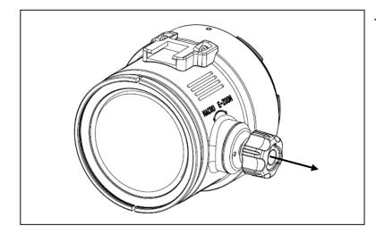
Make sure the control knob is at its most outwards position before mounting/ un-mounting the port. The knob should be left at this position until making sure that the lens and zoom gear is properly installed.
