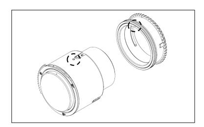
Align the inner groove of the macro switch gear with the white dot on the zoom gear tube. Then lightly push the gear towards the lens until it cannot go any further.
