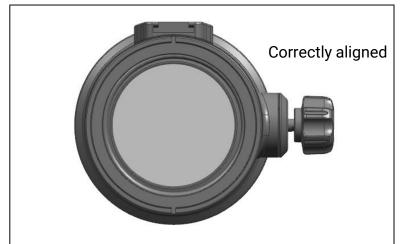
2. When properly installed, the lens should be perfectly concentric with the port. If there is a slight misalignment, check the position of the camera.
