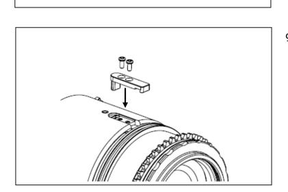
\*When mounting the Olympus 12-50mm EZ lens with the gear on the GH5/EM1X camera, or when removing them, the lens must be set to the "Macro" position.
