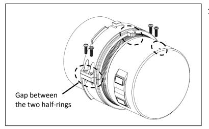
2. Align the alignment index on the ring with the dot on the lens before tightening the four screws. While tightening the screws, make sure that the gaps on both sides are even and the ring does not slip when turning at E-ZOOM mode.
