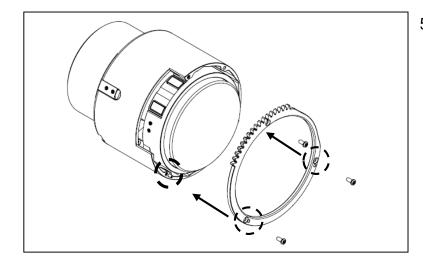
5. Align the pins on the tube with the holes in the gear ring as indicated in the diagram. Then tighten the three screws.
