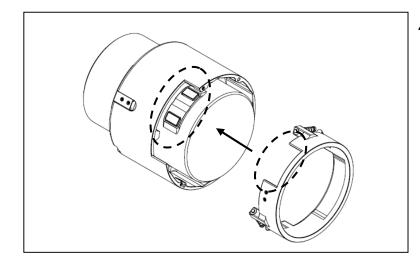
4. Align the spring ring with the lens as indicated in the diagram. Then lightly push the ring towards the lens until it cannot go any further.
