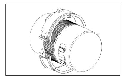
1. Mount the two half-rings on the lens zoom ring as indicated in the diagram.
