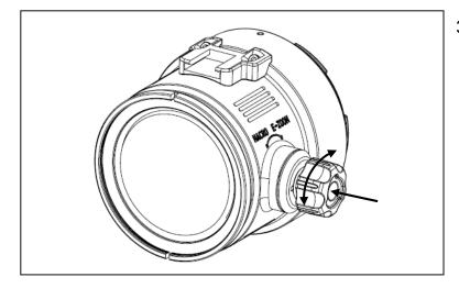
3. Engage the gear by pushing in the knob, then turn the knob for about 45° both ways to check if the camera switch between normal mode and Macro mode.
