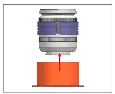
2 Insert the X1855-Z Zoom Gear on the plastic C-ring until it reaches the flange of the plastic C-ring.
