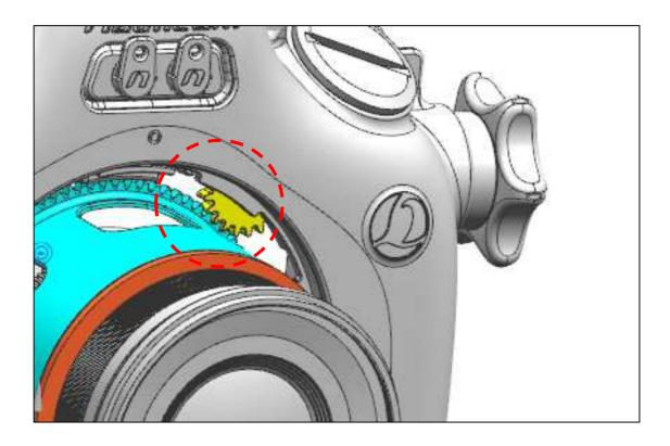
1. The X1024-Z Zoom Gear can be controlled by zoom/focus knob of the housing.
