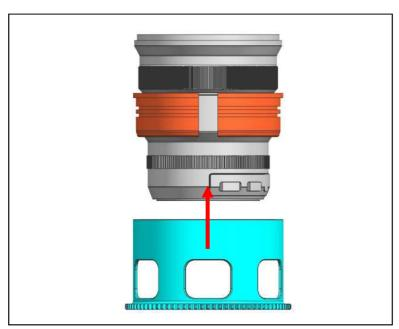
2 Insert the X1024-Z Zoom Gear on the plastic C-ring until it reaches the flange of the plastic C-ring.
