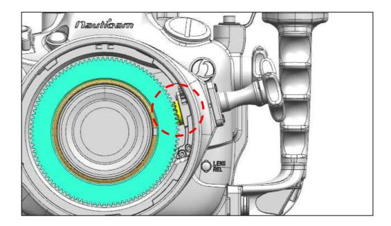
1. The SFE2860-F Focus Gear can be controlled by a focus knob of #37305 N100 to N120 35.5mm Port Adaptor II
