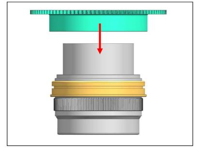
1. Insert the plastic C-ring as shown and place it over the lens.
