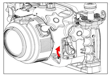
3. Lock the port into place by turning the port locking lever of the housing to the inward position. To ensure that the port is securely mounted, confirm that the green line on the safety button of the port locking lever is visible.
