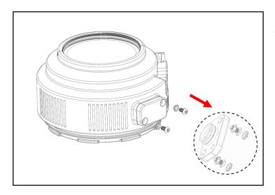
2. Remove the screws and focus knob plug from the port
