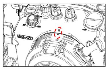
2. Align the "O" mark on the port with the WHITE dot on the housing. Gently push the port towards the housing until it cannot go any further.
