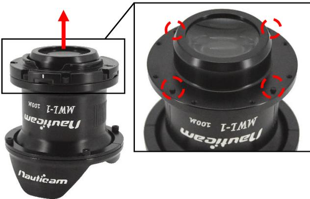
Remove the bayonet mounting ring of MWL-1. Note that there are 4x small black cylindrical positioning pins. All 4 pins should remain in the back of the lens
