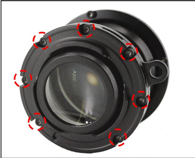
Remove the 7x screws from the back of the lens.
