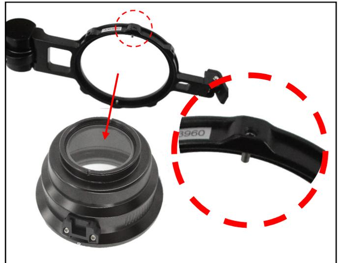
Align the two positioning screws on the back of the holder with the slots on the front of the port.
