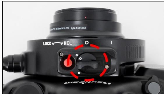
3. Lift the Port lock/ release latch on the other side of the adaptor. Then Press and hold the RED port release safety button, turn the port lock/release latch clockwise until it stops.
