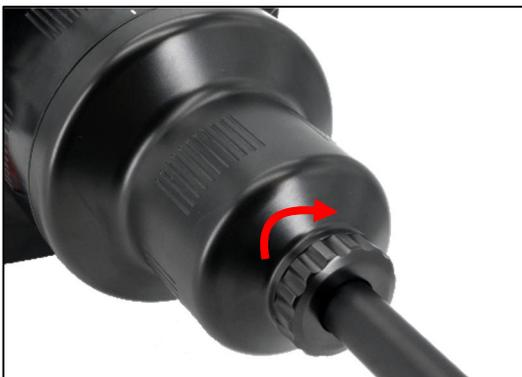
9. Fasten the locknut to squeeze the inside O-ring as well as grasp the lens for sealing
